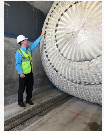
John Fortune, DHS S&T, points out features of the Resilient Tunnel Plug at a demonstration for media. Quick inflation and extreme strength of the plug's material hold back water that might enter a subway tunnel during a flood. Credit: DHS
