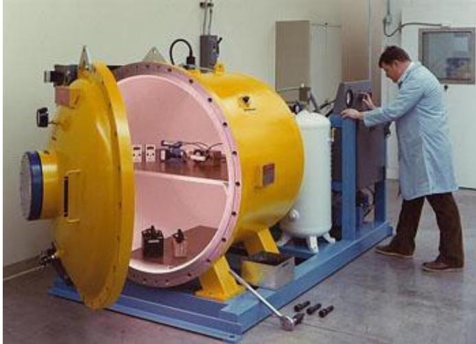
PNNL researchers test performance of commercially available radiation detectors with equipment such as this pressure chamber.
