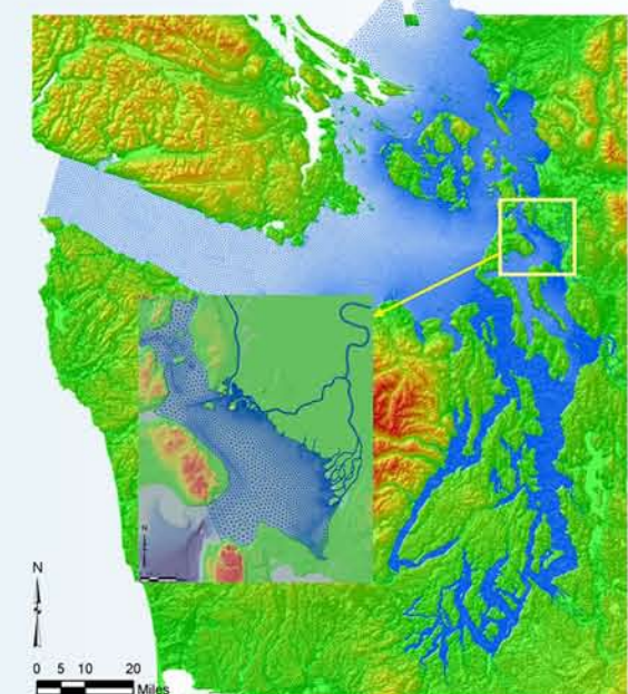
Hydrodynamic Model Grid for Puget Sound Used by PNNL - Puget Sound Model. The inset shows detail for the Skagit Basin.
