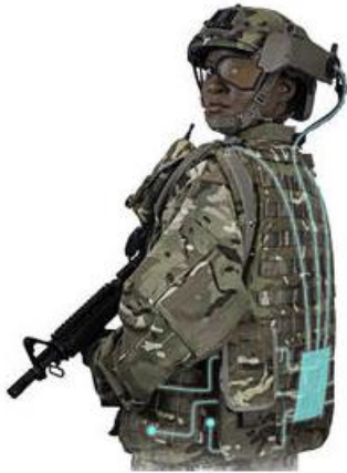
A soldier wearing the BAE Broadsword power and data distribution harness, which uses e-textiles embedded within the uniform.
